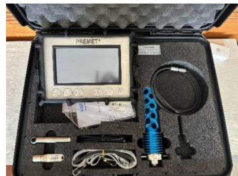
Figure 17. In-cylinder pressure sensor analyser.
