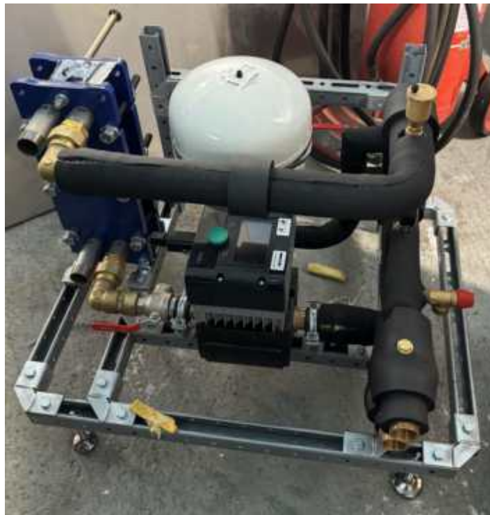
Figure 15. Fresh water/glycol circulation loop.
