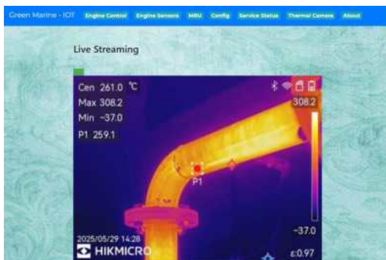
Figure 5: Thermal camera live stream from IoT.
