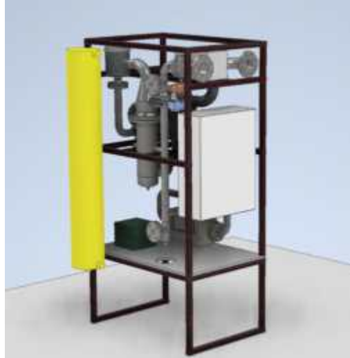
Figure 14. Main equipment skid, flue gas conditioning, HX-1; flue gas fan, P-2; Separaptor unit, SEP-1, Membrane unit Mem-1 (yellow), Permeate vacuum pump P-3; and control cabinets. Flanges at the top of the skid show hot flue gas feed entering to the right and to the left is the return flange for the mixture of CO 2 -depleted retentate and CO 2 -enriched permeate from the membrane module.
