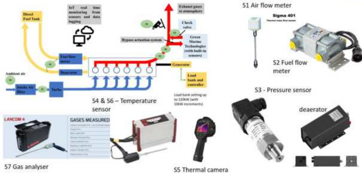
Figure 1: Latest land-based test setup with sensor location.
