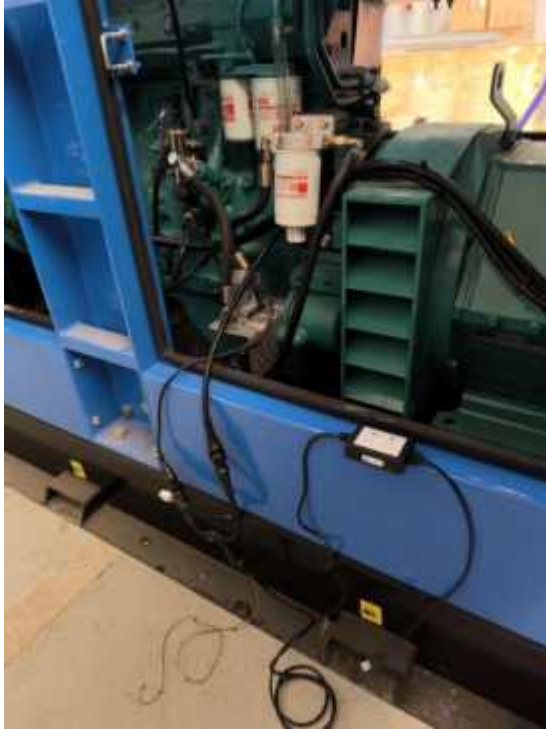
Figure 8. Fuel and air flow meter sensors connected to IoT Raspberry Pi5 (CanBus) and ECU (ModBus RTU) respectively. The flow meters have also been calibrated.
