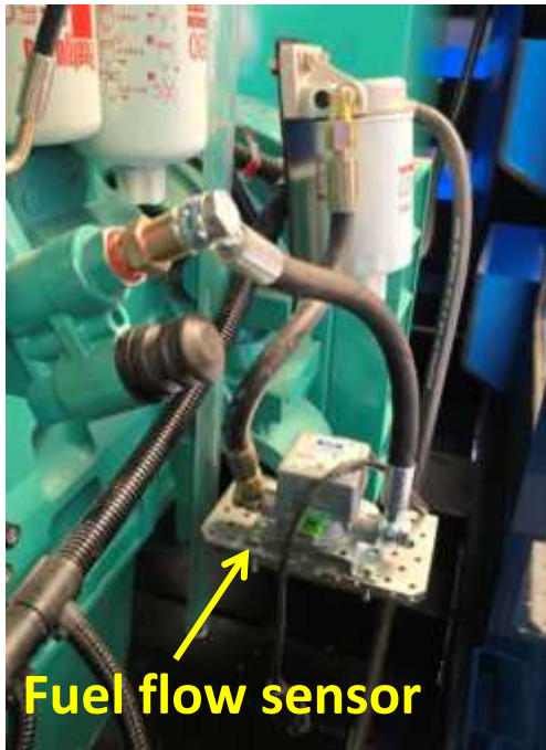
Figure 5: Left: Installation of fuel flow sensor on the marine genset. A plate was used to support the fuel flow meter. Right: The integration of the sensor was setup as per the fuel flow meter manufacturer's instructions.
