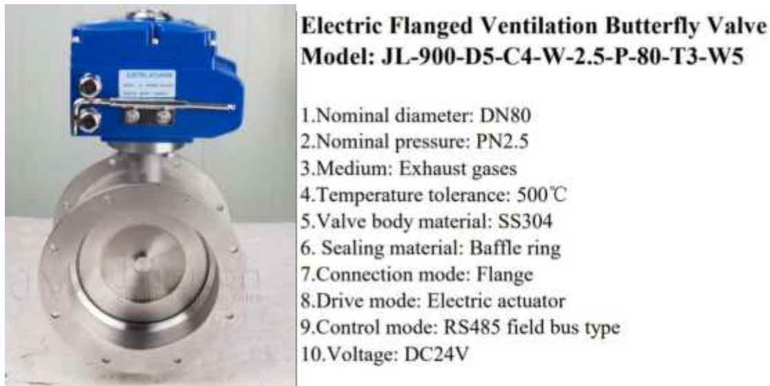
Figure 19. Electrically actuated bypass valve (left) and specifications (right).
