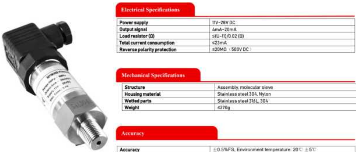
Figure 21. Left: RS PRO Pressure Sensor, 0 bar Min, 4 bar Max, Gauge Reading. Right: Electrical, Mechanical specifications and accuracy.
