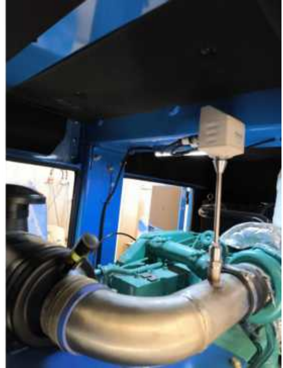
Figure 8. Fuel and air flow meter sensors connected to IoT Raspberry Pi5 (CanBus) and ECU (ModBus RTU) respectively. The flow meters have also been calibrated.
