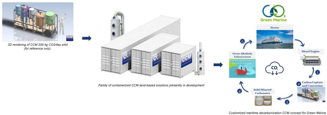
Figure 1. The standard CCM process and design will be customized for maritime applications.
