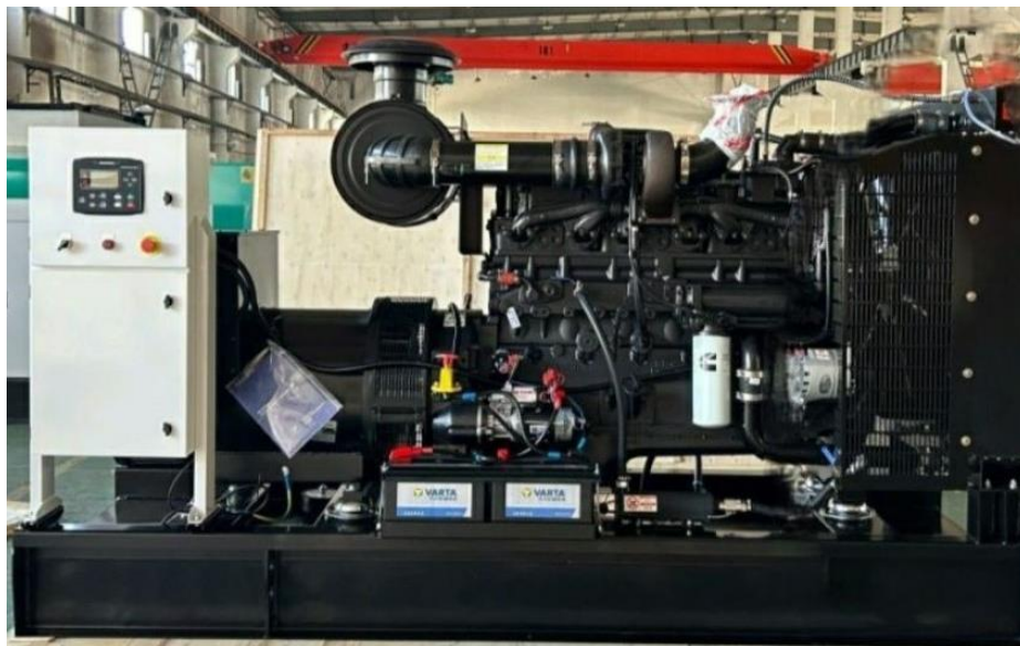
Figure 5: Marine genset for land-based testing.
