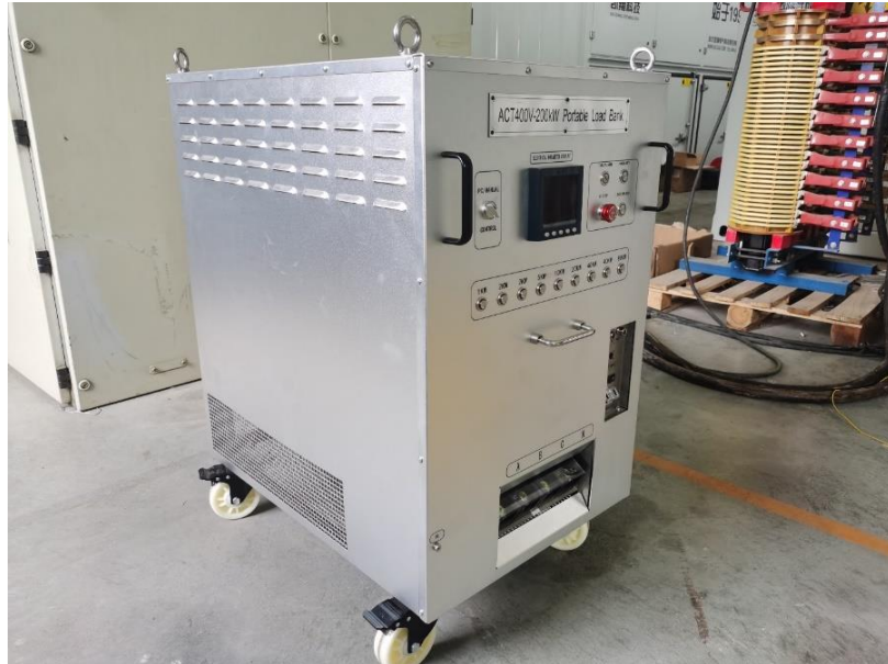
Figure 6: Portable load bank for land-based tests.
