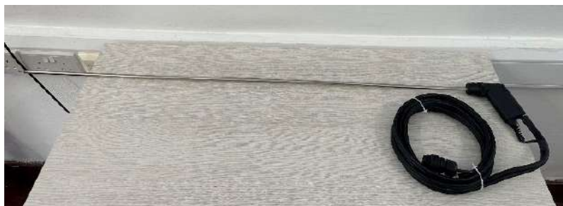
Figure 2. Smoke detector connected to Lancom 4 Gas Analyzer
