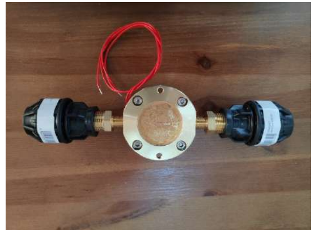
Figure 4. Fuel/oil flow meter
